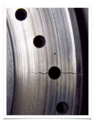
when cracks between multiple holes connect, which can lead to a large chunk of rotor breaking free. Not a pretty sight.
