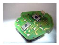
The remote itself may be damaged. When a door doesn't immediately open upon depressing the button, what do we do? We press harder! After multiple times the delicate circuitry in the remote may break a line or a component may just die.
