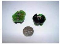
lid, etc. The remote control uses a common, 3 volt button battery which needs to be replaced every few years. The battery model is 2032.
