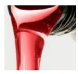
light oil, generally red with a strong petroleum smell, but if it's overdue for replacement it's dark brown in color and may smell burnt. Manual tranny fluid in Porsches is very viscous - much heavier than motor oil - has a deep blue or green color and smells like rotten eggs.
