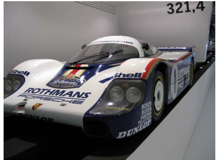
956/962 cars were the first ground effects cars from Porsche—enough downforce to drive upside down
