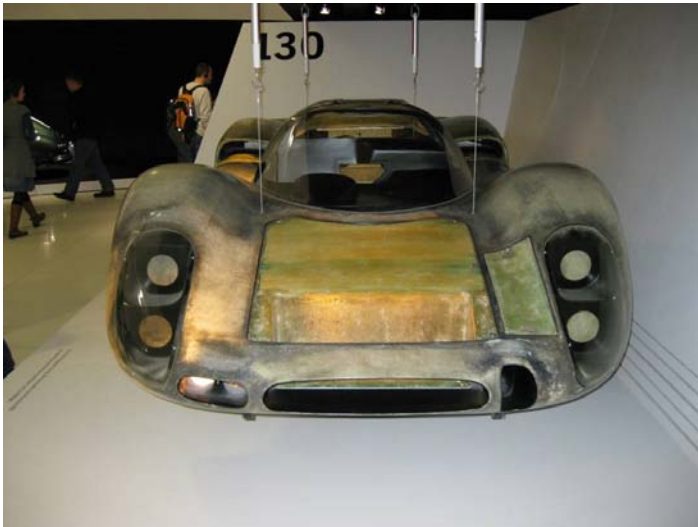
917 Body, so thin that light shows thru the fiberglass
