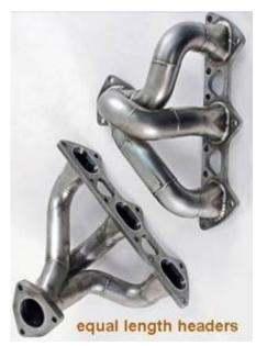
What makes the headers work is that they help to eliminate back pressure. Instead of having all three cylinders on one side of the engine share one common exhaust manifold, with headers, each cylinder gets it's own exhaust pipe.
