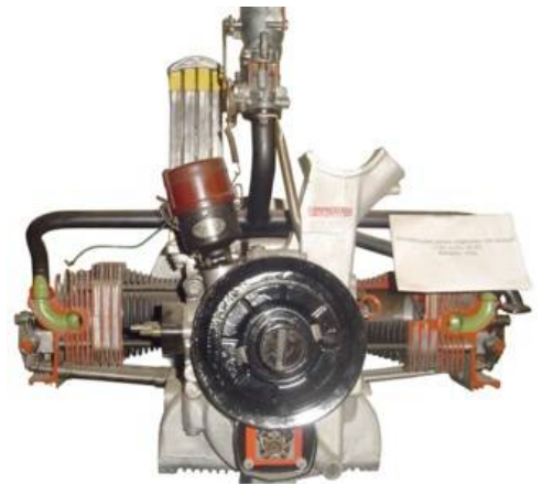
1945 VW engine cutaway
