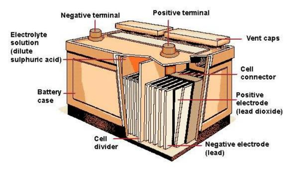
Starter batteries are made up of many thin lead plates which enable them to discharge a lot of energy very quickly which is what's required by a vehicle's starter motor which must turn over the engine in order to start it.
