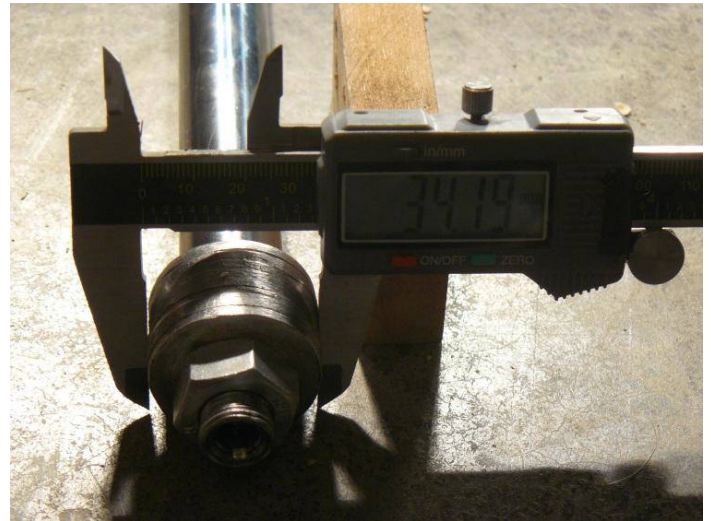
Outside Diameter of Washer Stack = 32.4 mm
