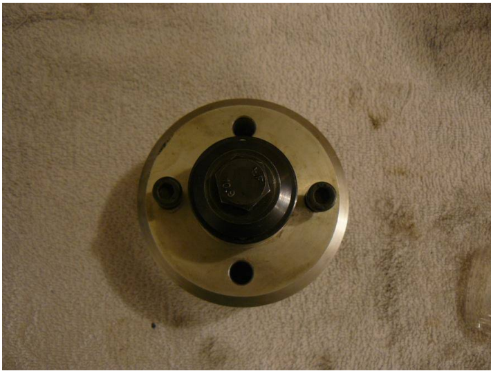
VW Tool used to insert the new rear main seal
