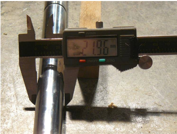
Outside Diameter of the Shaft = 22mm
